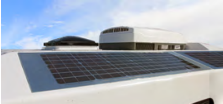
Photo above is a 90W Super Thin solar panel bonded to caravan roof.
